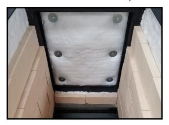
Finished bricking. Backside of the front door frame.
